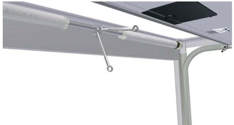
Whilst holding this light tension, place the centre torque clamp on square portion of shaft and secure to bracket with two nuts.
