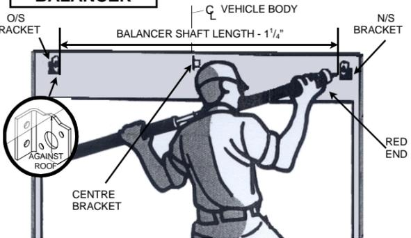
Find centre line of body and mark end bracket positions (see diagram.) Weld or bolt brackets as close to roof as possible. Insert balancer with red end on the right (viewed from inside the body.) Insert split pins on either side of right hand bracket and open out to retain in position.
